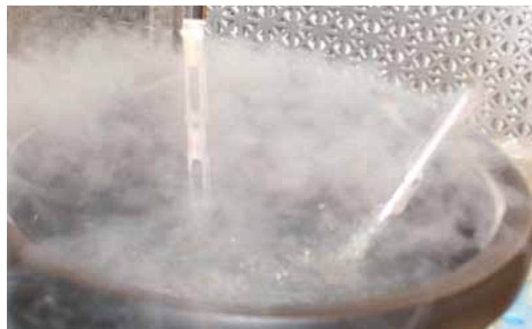
Cassava cryopreservation experiment: sample cooling in liquid nitrogen. Photo by IITA
