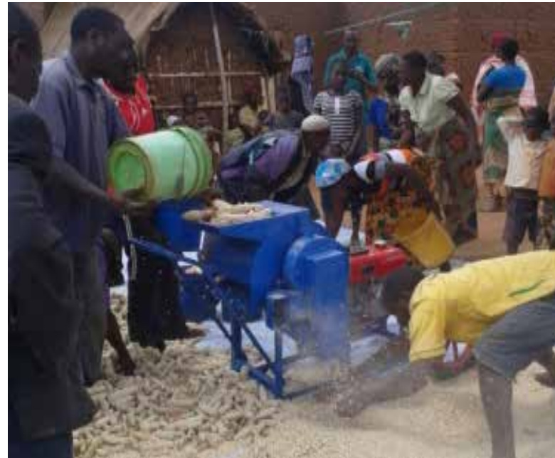
Farmers using the motorized maize-shelling machine at Yohana Isaya’s farm during a postharvest training organized by the Africa RISING – NAFKA scaling project in Ndurugumi village. Photo by Francis Muthoni, IITA.
