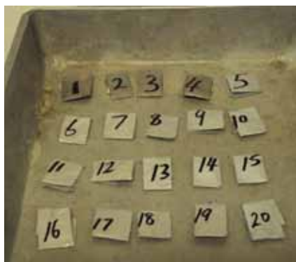
Figure 12. Seed samples in aluminum foils for oven drying.
