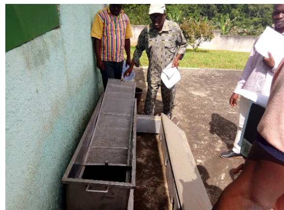
Components of the rectangular steamer
