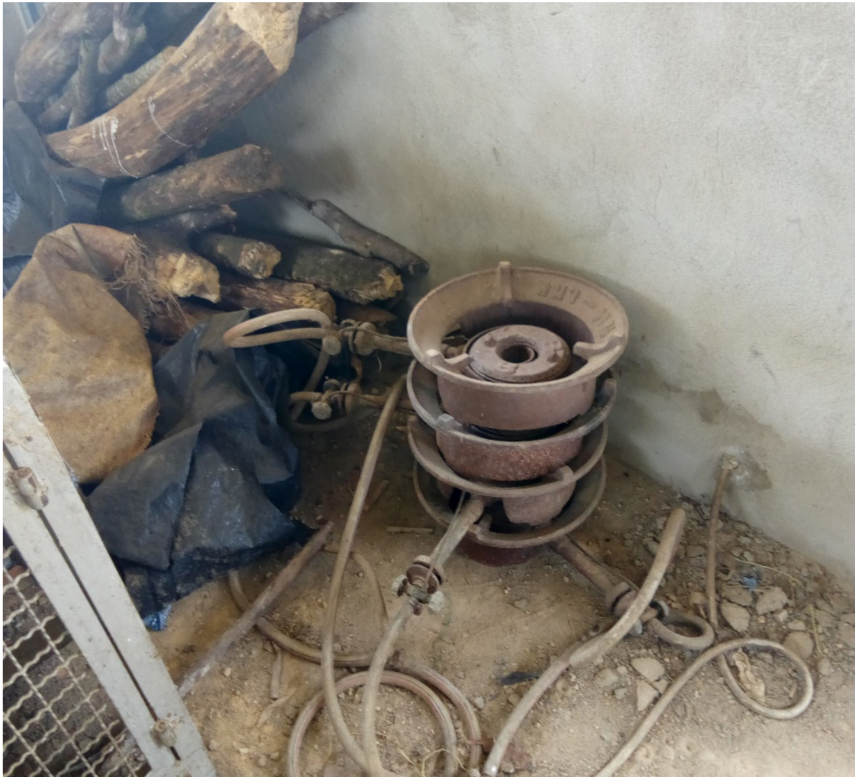
Plate 11. Gas-fired burners for steamers set aside. Source 2018 Field trip
