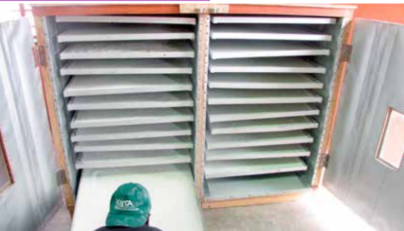
Loading trays laden with wet cake particles into the steam dryer cabinets. Photo by Braima James, IITA.
