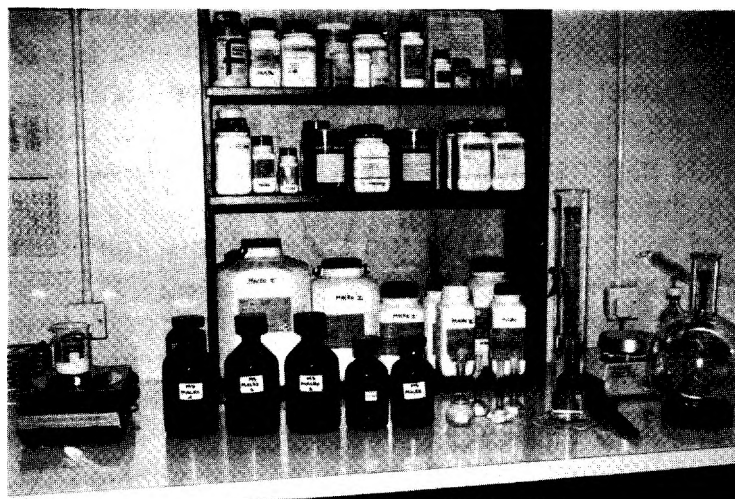
Figure 3. Medium preparation from stock solutions. From left to right: balance with sugar being weighed, MS mineral salt stock solutions in dark bottles, vitamin and growth regulator stock solutions in volumetric flasks, graduated cylinder with distilled water, pH stick, boiling flask.
