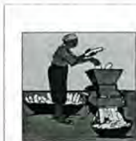
Convey the washed tubers to a mechanical grater. Discharge the grated cassava into a clean container or directly into bags made of polypropylene.
