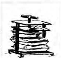
The water drains out through the holes in the polypropylene socks during the fermentation stage. To remove moisture use a power screw shaft. (Moisture content is about 50%)
