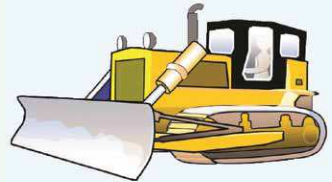
Figure 16 : D6 light bulldozer
