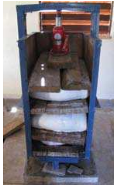
A hydraulic press used to remove excess water from cassava mash
