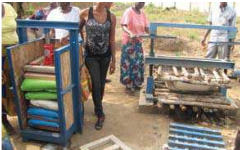
A hydraulic press (left) or screw press (right) (here they are on display outside the factory)
