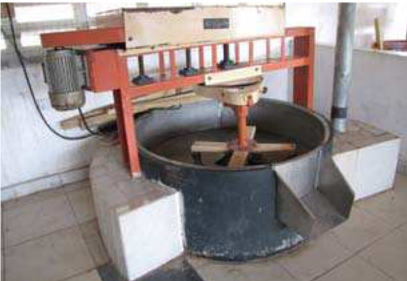
An automatic gari roaster is ideal for producing large volumes of gari
