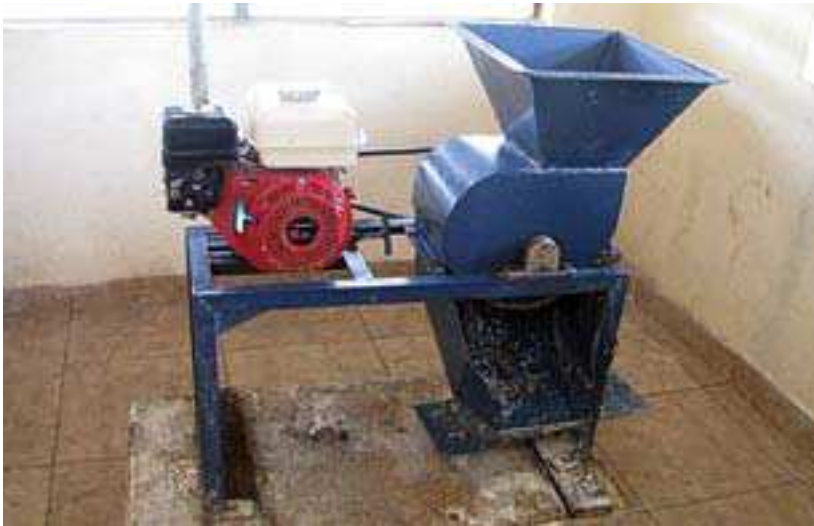
A motorized grater used to crush cassava roots into a wet mash
