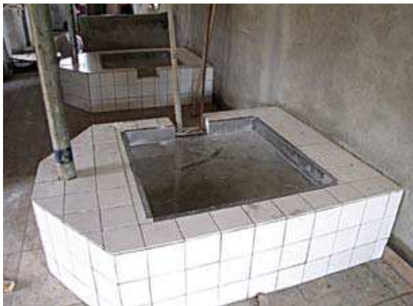
A gari roasting bay with a shallow stainless steel tray or a moulded aluminium pot. The tray should be mounted on simveram or mud bricks rather than cement bricks, since these are more heat efficient. The tray should have a tiled surround so the area can be kept clean.
