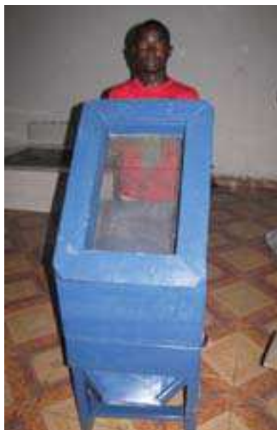
A gari sieve made from stainless steel mesh
