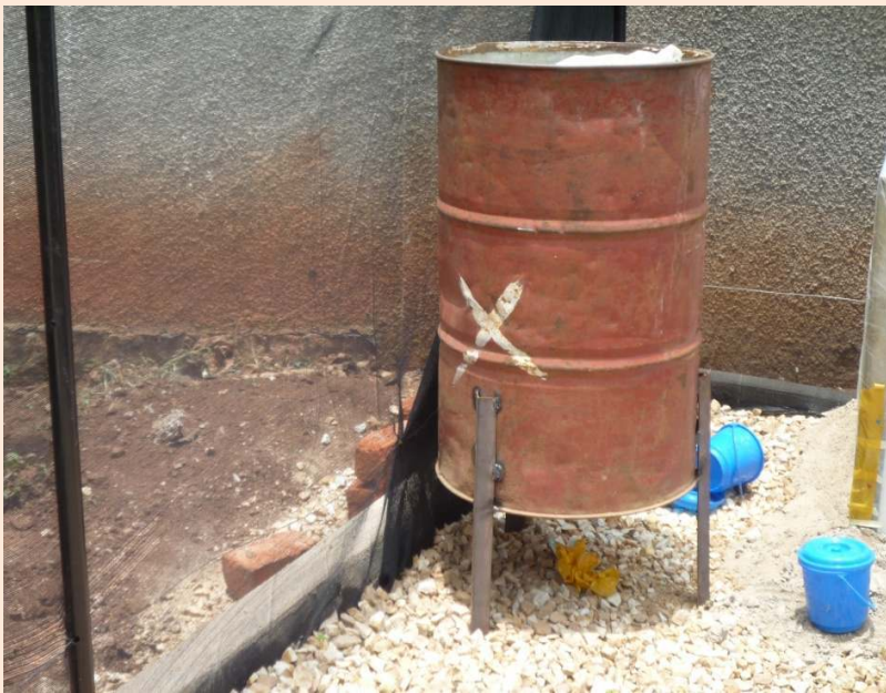
Fig. 6. Oil drum used for heating the soil mixture.
