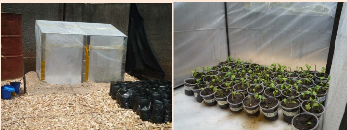
Fig. 2. A medium-cost humidity chamber made by wrapping polythene sheeting around a metal frame.
