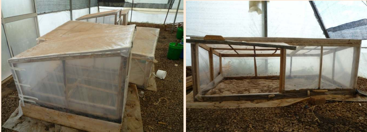
Fig. 3. A medium-cost humidity chamber made by wrapping polythene sheeting around a timber frame.
