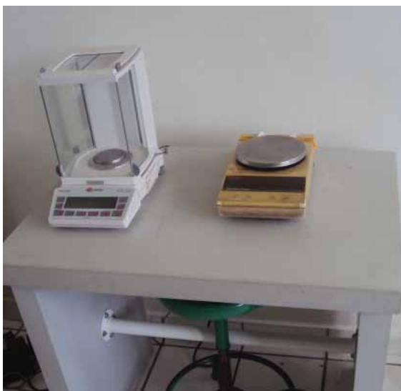
Photo 4. Sensitive weighing balance (left) and the “g” one, on the shake-proof table.
