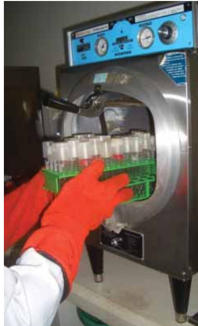
Photo 6. Sterile medium taken out from the autoclave, after completion of the sterilizing cycle.
