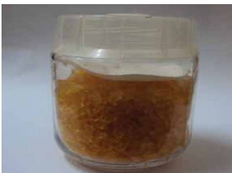
Photo 57. Physical dehydration: Baby food jar filled up with silicagel and cover by a filter paper.
