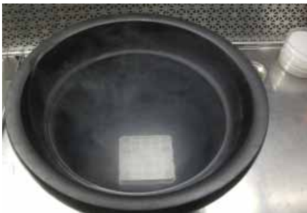
Photo 49. Cryovials (in rack) immersed in LN, containing the aluminium strip carrying PVS2 droplet with the meristems.
