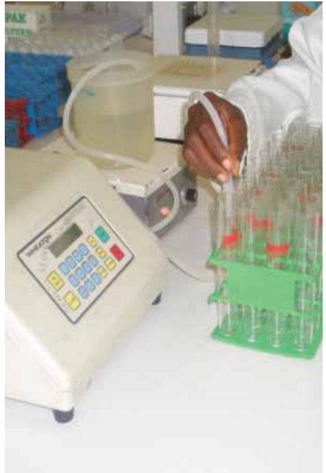
Photo 11. Culture medium dispensing using automatic media dispenser
