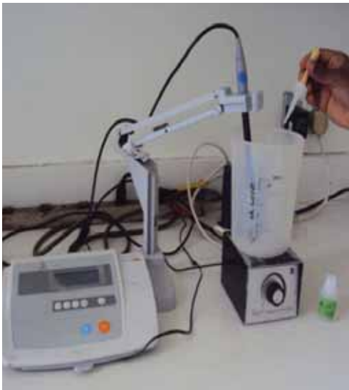
Photo 10. pH adjustment using pH-meter and magnetic stirrer.
