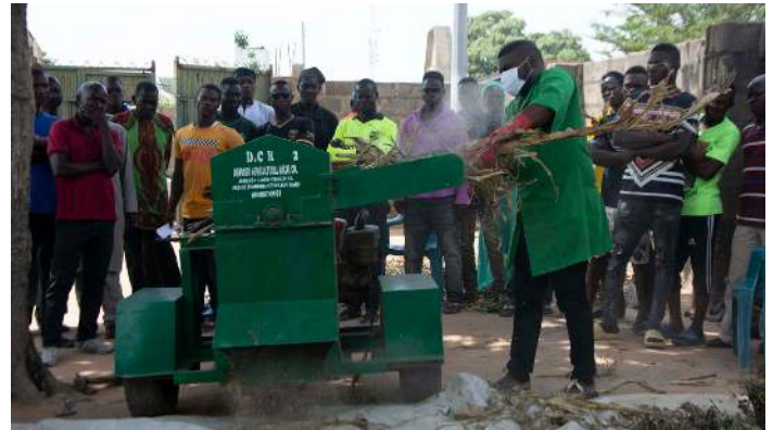
Activity Staff, Leke Balogun shows training participants how the Stover Crusher works.
