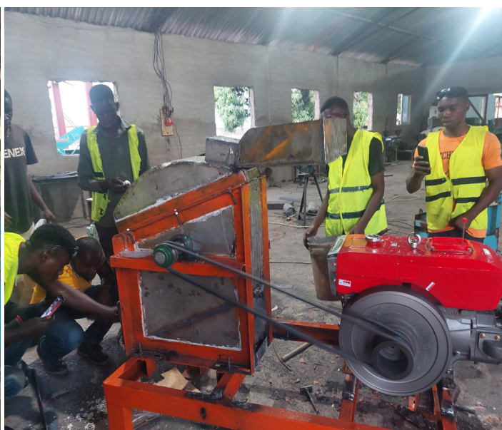
Left: A trainee practicing how to cut the stainless steel sheets. Right: The trainees testing the completed Wet Hammer mill.
