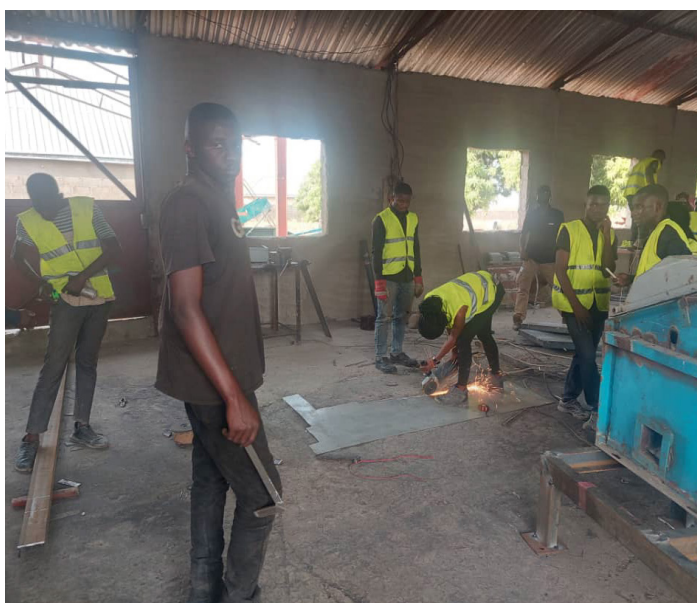
Left: A trainee practicing how to cut the stainless steel sheets. Right: The trainees testing the completed Wet Hammer mill.
